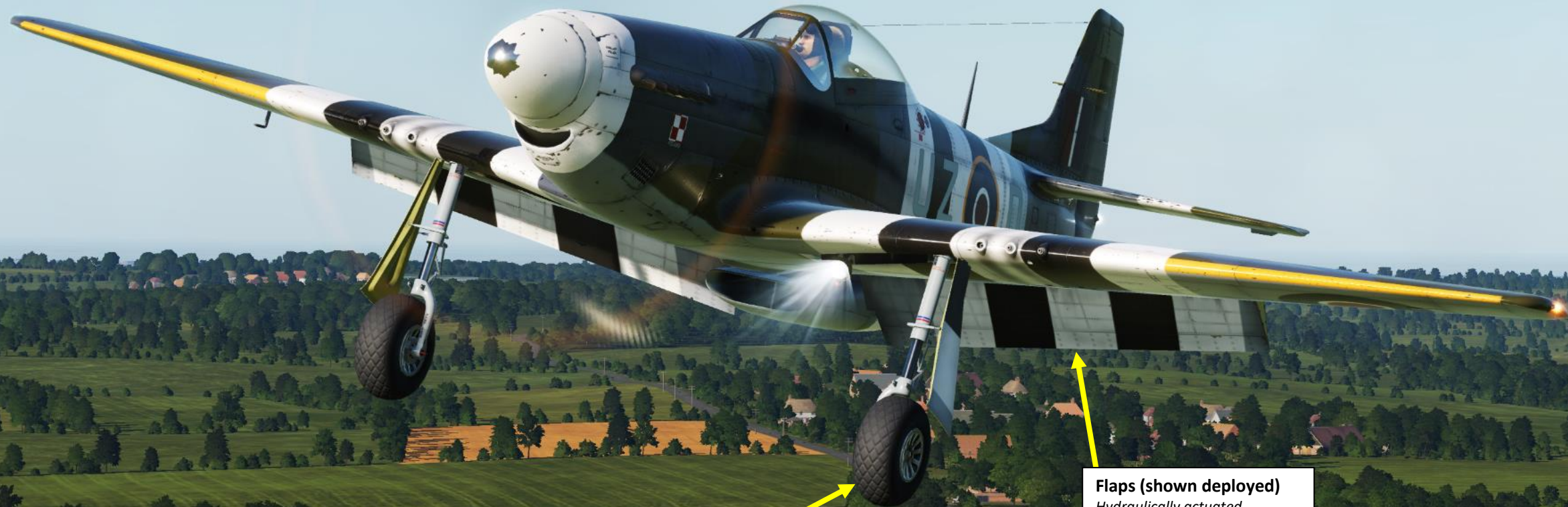
Landing Gear (shown deployed) Hydraulically actuated
